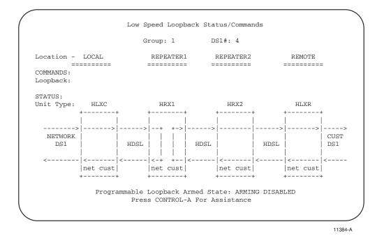
Figure 541-9a. HRX1 Customer Loopback Screen (Two HRXs)
